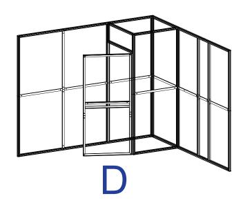
3. Attach module D as illustrated in the diagram.
