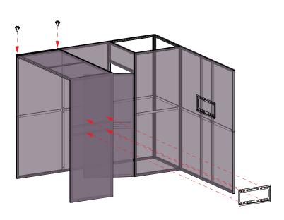
5. Attach module F to the main structure, and then mount another TV rack onto module D.
