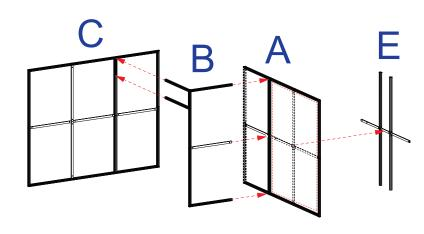
2. Then, connect modules A, B, and C together to form a booth. If you plan to install the screen monitor, replace the "cross frame" (dot line part ) inside module A with module E.
