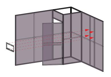
4. Install the front and back graphics, then mount one of the TV racks onto module A.
